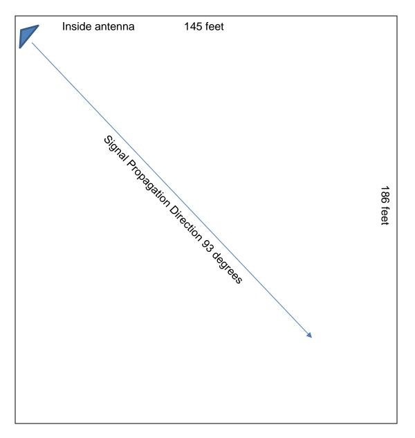
Directional antenna transmits signal towards opposite corner. Signal outside hangar at 100 feet: less than -140dBm.
