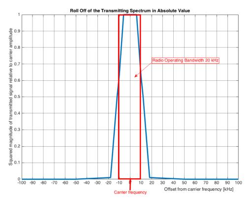
In the uplink (ground station to CubeSat), a Universal Software Radio Peripheral (USRP) B200 software defined radio from Ettus Research will be used with directional antennas and power amplifiers to deliver a transmit power of 13.98 dBW (25 W). A similar roll-off characteristic for the transmitting spectrum is assumed in the uplink, which can be easily implemented as a digital root-raised cosine (RRC) filter in the B200 USRP.
