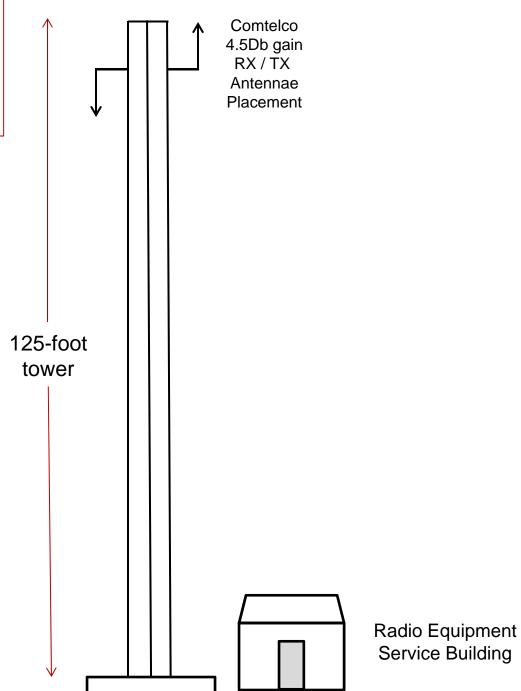
Sketch supporting FCC License Comtelco 4.5Db gain application 0696-EX-CN-2016 RX/TX (FAA Sketch) Antennae Chilocco Indian School Campus **Placement** 36° 59' 16"N 97° 04' 07"W 75-foot tower Chilocco Security Building/ Radio Frequency Range Control Room
