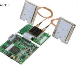
The SDR processor module SDR-PM 402 is compatible with this SDR-RF 980B module. The graphic user interface software SDR-GUI is for activating this RF module, selecting operation parameters, and collecting data.
