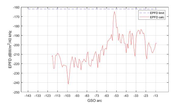
As seen by the plot above, the GETSAT operations are compliant with the EPFD ↑ limits in Article 22 of the ITU Radio Regulations.<sup>3</sup> This graphic is for when the antenna boresight is pointing toward an O3b satellite located at 55°W.
