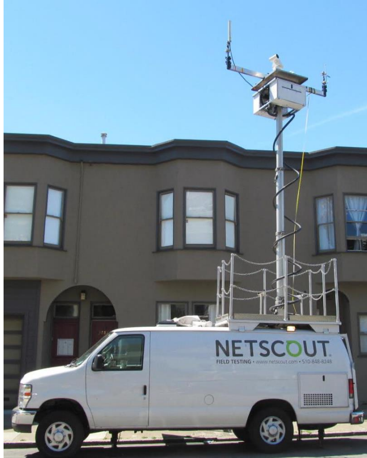
Figure 1 - Mobile transmitter unit for CW testing. Maximum height for telescoping mast is 15m.
