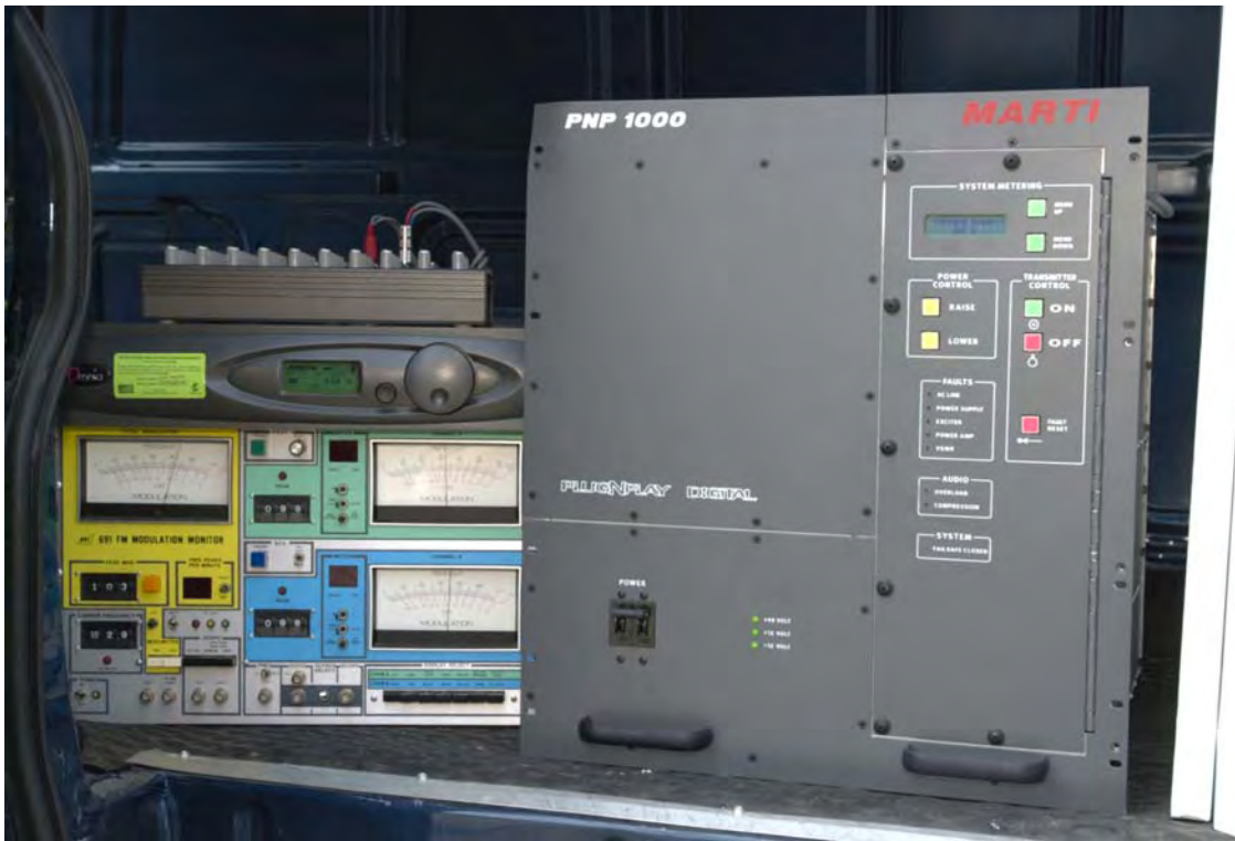
Mixer, stereo generator, modulation monitor and FM transmitter operating in the van.
