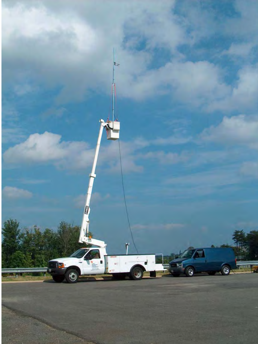
Bucket truck with antenna deployed, van with electronic equipment and generator set up near The George Washington University Prince William Campus.
