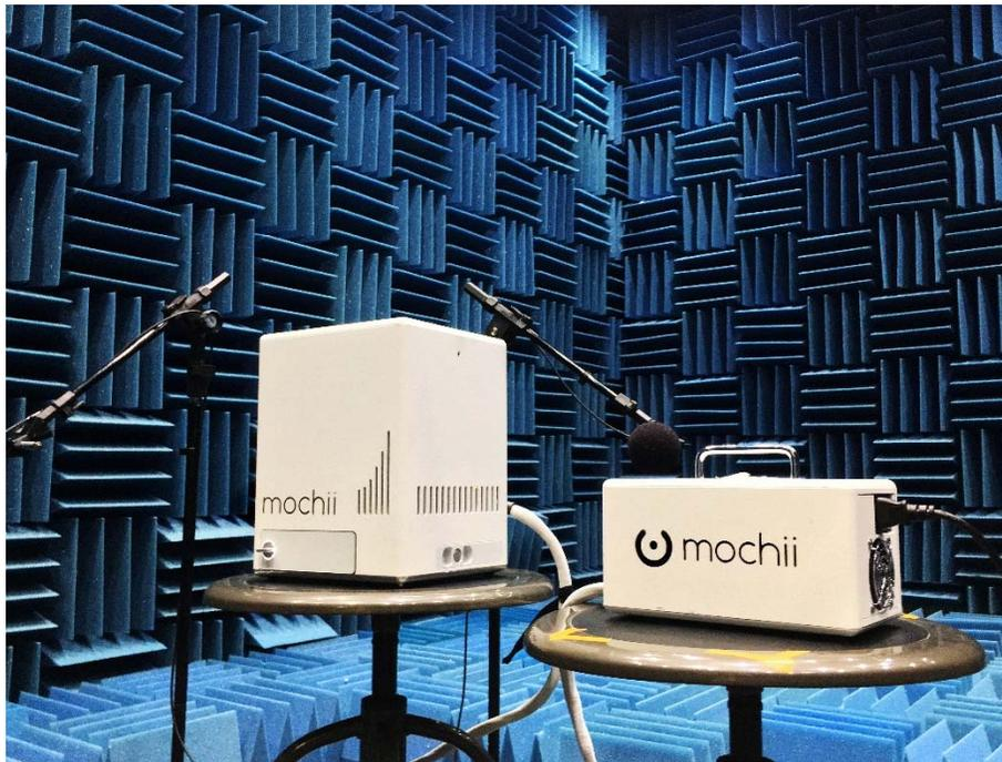
Mochii, Inc. (DBA Voxa) has been working with NASA to certify Mochii for operation aboard the ISS. Mochii has undergone rigorous testing including EMI/EMC certification testing at Johnson Space Center. The flight-certified Mochii was flown up to ISS on the Northrop Grumman NG-13 commercial resupply mission on February 15th, 2020. Mochii will provide NASA the capability to analyze samples in on-orbit microgravity experimental conditions without having to send them back down to earth.
