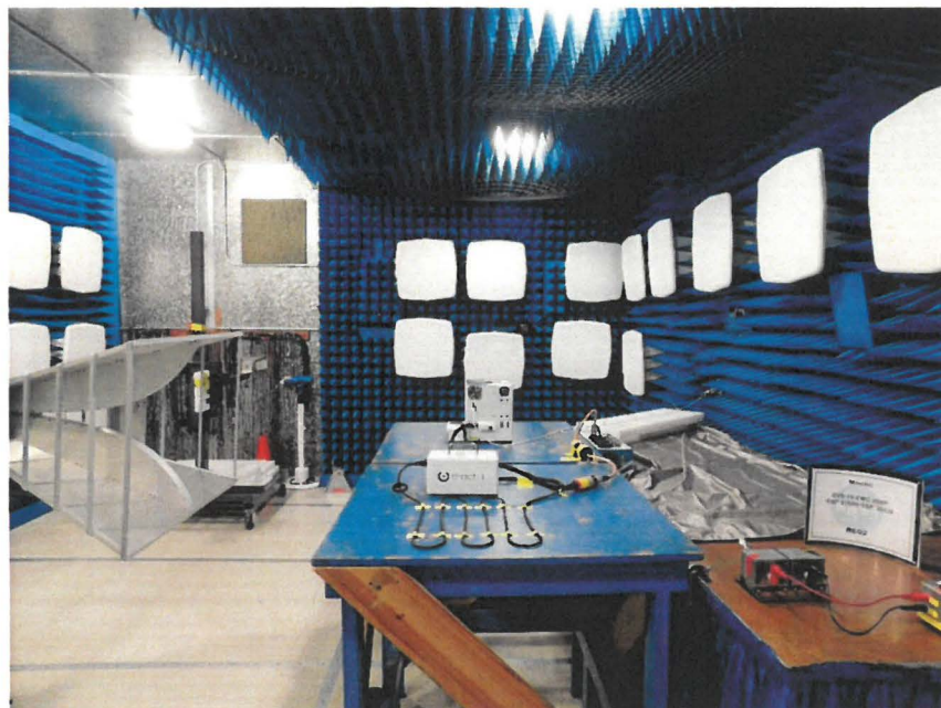
Figure 4.1.7.4: RE02 Test set up – Semi anechoic chamber, Horn Antenna Vertical Polarization, 200 MHz – 1 GHz
