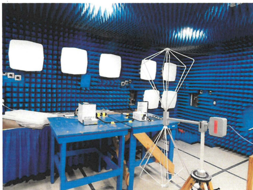
Figure 4.1.7.2: RE02 Test set up – Semi anechoic chamber, Biconical Antenna Vertical Polarization, 100 MHz – 200 MHz
