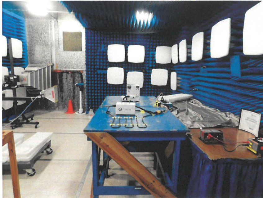
Figure 4.1.7.5: RE02 Test set up – Semi anechoic chamber, Horn Antenna Horizontal Polarization, 1 GHz – 15.5 GHz
