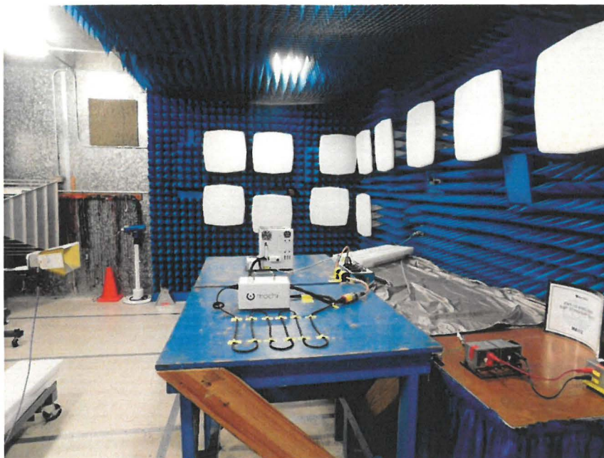
Figure 4.1.7.6: RE02 Test set up – Semi anechoic chamber, Horn Antenna Vertical Polarization, 1 GHz – 15.5 GHz
