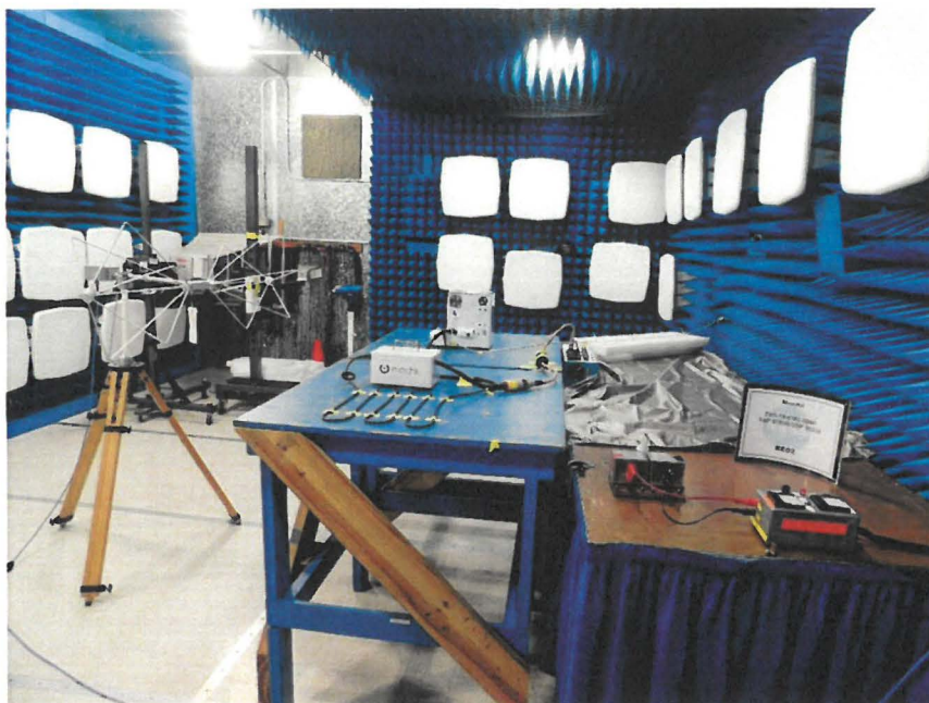
Figure 4.1.7.1: RE02 Test set up – Semi anechoic chamber, Biconical Antenna Horizontal Polarization, 100 MHz – 200 MHz
