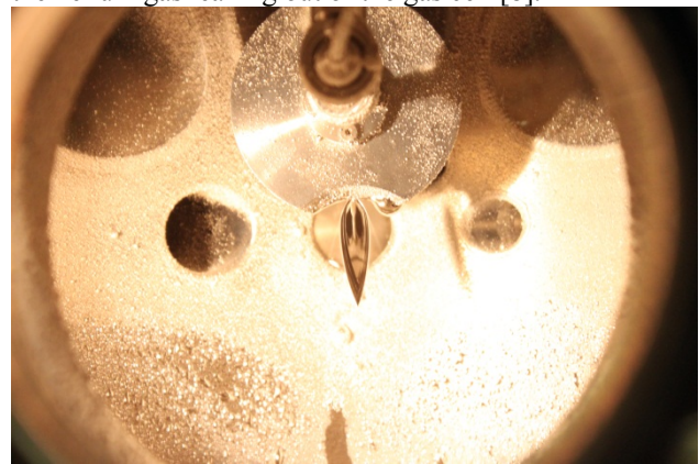
Figure 3: Liquid lithium film established at ANL.
