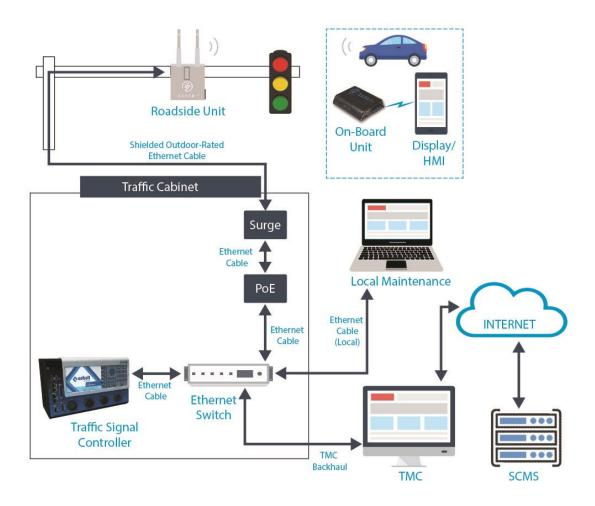
Figure 2: Signal Phase and Timing (SPaT) Messaging Diagram
