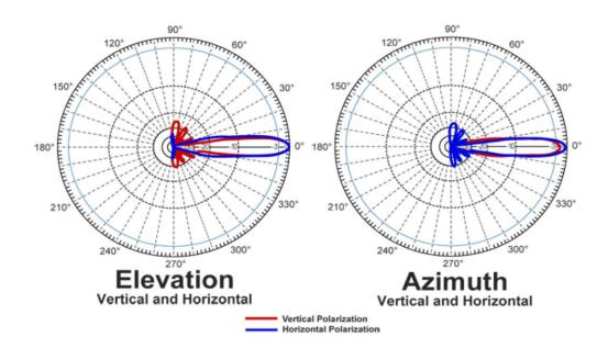
The beam pattern for the S-band dish antenna is shown below. The 3dB beam width is 8.4deg.
