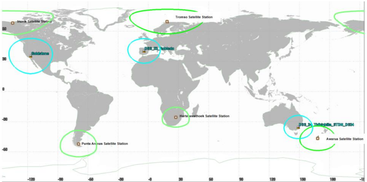
Figure 2.f.4. Transmission footprints from 275 km for contact with mission ground stations. Sub-satellite footprints for contact with the AMS ground stations (in green) and their potential overlap with DSN stations (in blue).
