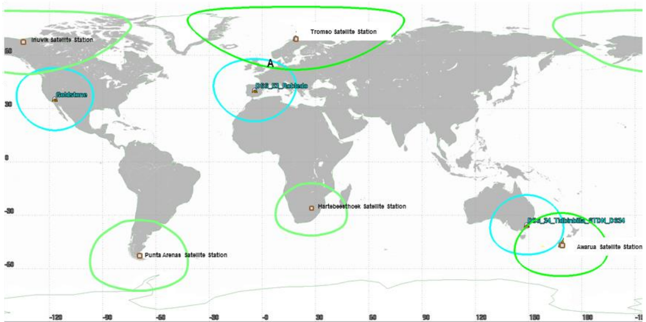
Figure 2.f.3. Transmission footprints from 500 km for contact with mission ground stations. Sub-satellite footprints for contact with the AMS ground stations (in green) and their potential overlap with DSN stations (in blue). Point "A" indicates location analyzed for potential DSN interference.
