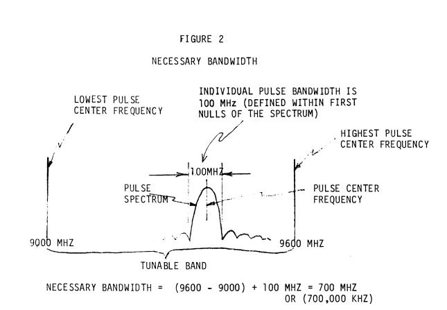
(The necessary bandwidth is equal to the tunable bandwidth, i.e., 600 MHz, plus the 100 MHz modulation bandwidth).
