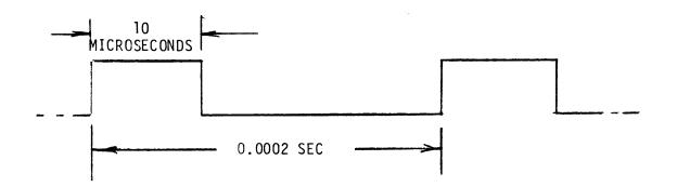
EACH 10 MICROSECOND PULSE IS BI-PHASE MODULATED WITH SUBPULSES OF 20 NANOSECONDS OR LONGER.
