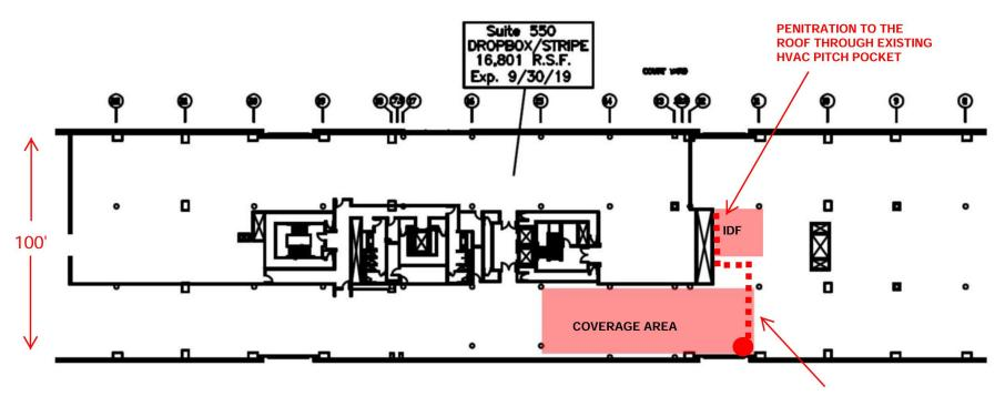
90 ft. LMR-400 cable connecting repeater to active antenna (mounted above IDF on roof)
