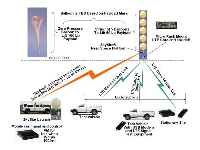
Space Data's proprietary NPCS 900 MHz data link (which will utilize NPCS 900 MHz spectrum licensed to Space Data) from the SkySite® Platform to the ground station will provide the ability to control the LTE transmitter over a wide area (out to 300 miles from the test truck). There will be no backhaul link from the LTE system on the SkySite® Platform as the Oceaus Networks Xiphos core will be flown as well.
