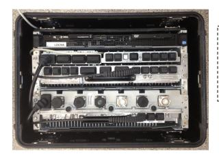
The LTE RAN is designed to provide macro coverage with up to MIM0 2 x 60W operation with up to 20MHz channel bandwidth — maximizing range and packet data throughputs with shared data throughput of 150Mbps per sector to subscriber handsets. The system is deployed quickly and simply providing operational coverage within 4 minutes of system switch on.
