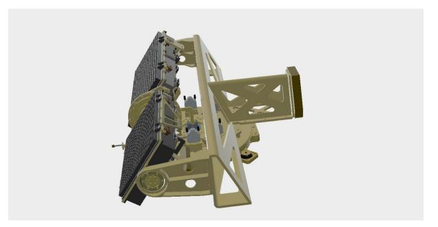
The TX array has dimensions of 11.5 inches wide by 7 inches high. The RX array has dimensions of 17.5 inches wide by 7 inches high. The supporting gimbal is a standard elevation over azimuth configuration.
