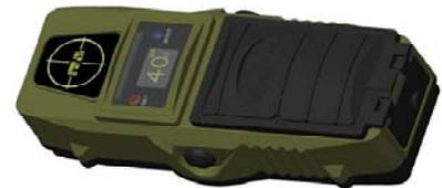
In use, the operator places the device against the wall of a structure and depresses the scan buttons. Within 1 second for moving targets, or 3 seconds for a stationary breathing target, the display shows the range to the nearest target.
