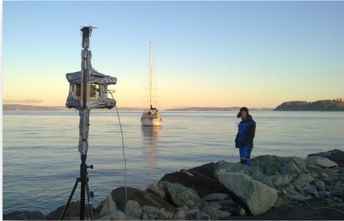
Testing flat sea fading on a freezing day in Trondheim, Norway
