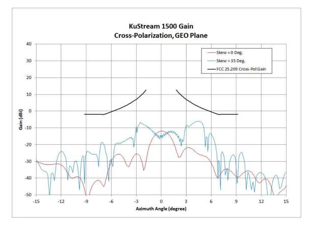
The terminal will be configured to not transmit more than 44 dBW EIRP. (This translates into an ERP of 15,310 W and a transmit power of 17.35 W). This power limitation is implemented as part of the commissioning procedure of the terminal.
