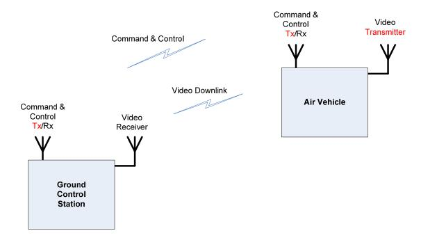
As part of the test capability, Honeywell is also testing an alternate video transmitter and receiver solution which integrates the L3 Communications radio operating in the 1700-1880 MHz range.
