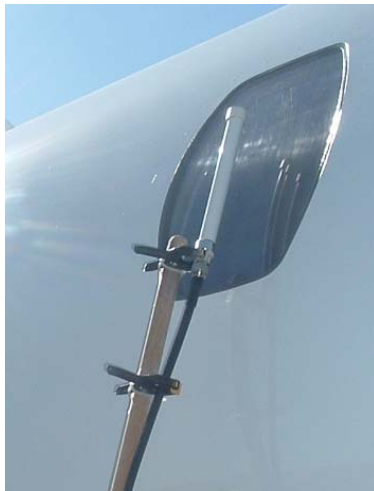
Figure 9. Typical outside PCS antenna location for ingress tests
