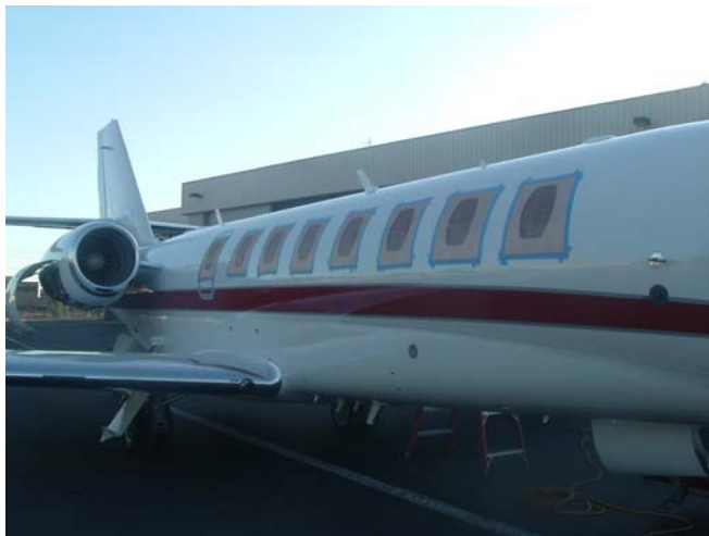
Figure 5. Shielding material fixed to aircraft
