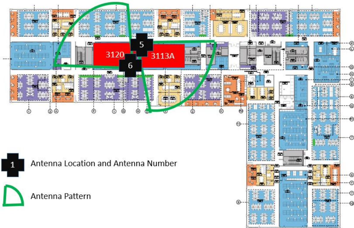
Figure 5 - Location of antenna in the HPI Facility – Third Floor test labs
