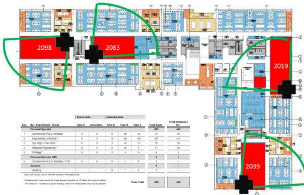
Figure 4 - Location of antenna in the HPI Facility – Second Floor test labs
