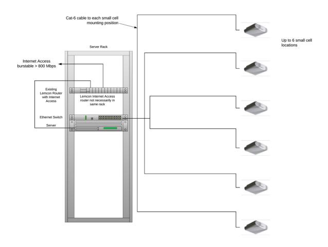
The CBRS small cells will be ceiling or wall mounted. Each small cell is expected to cover between 3,000 and 6,000 square feet. The main radio parameters of the equipment are:
