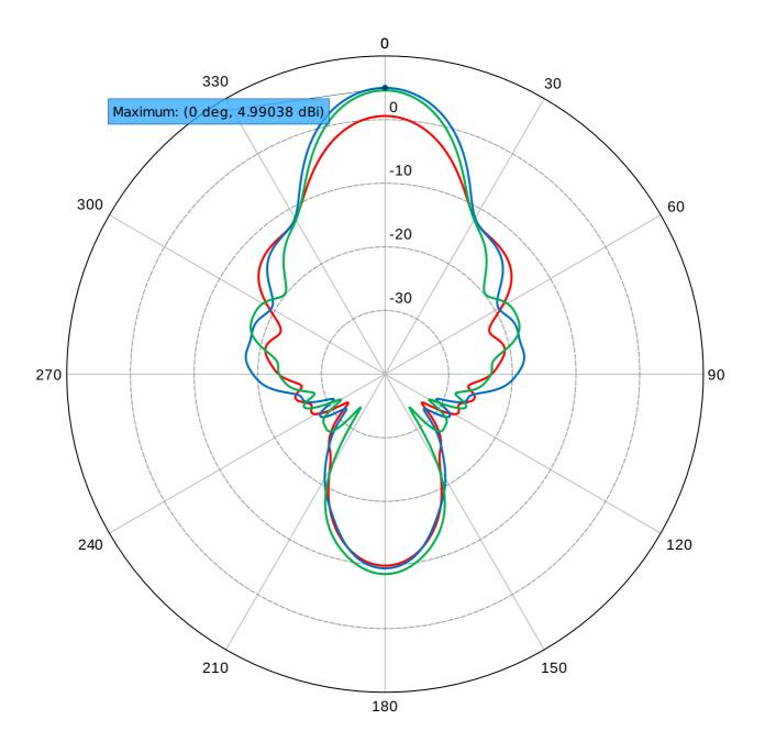
Total Gain (Phi' = 90 deg) - WR187\_Gain\_Horn
