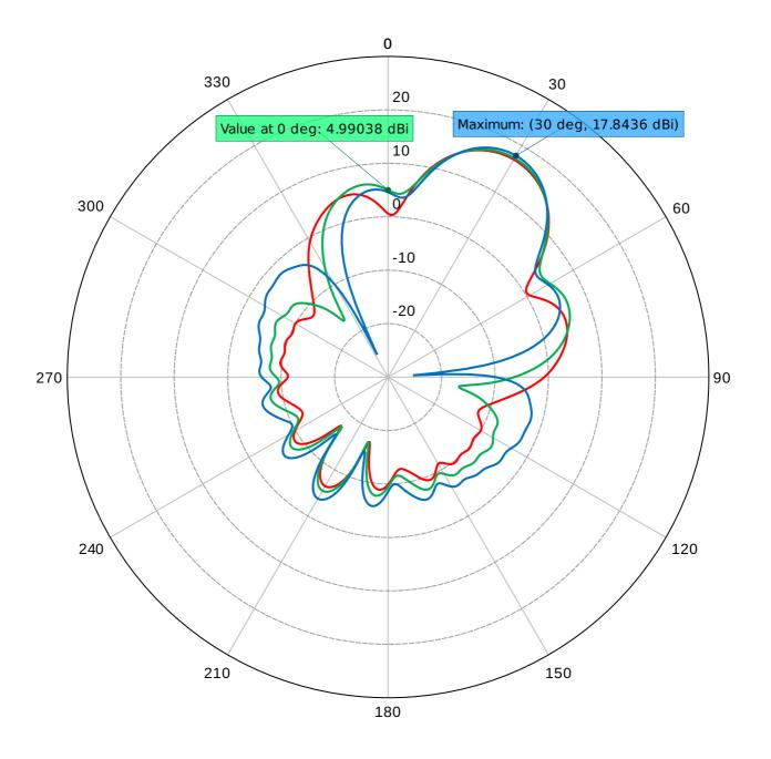
Total Gain (Phi' = 0 deg) - WR187\_Gain\_Horn
