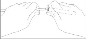
against opposite button insulator will help maintain center reference (if you push the first retainer too far, remove element from boom, push retainer completely off the element, and start over). Install another retainer to the opposite side of the element. Continue installing retainers until all elements are secured.
