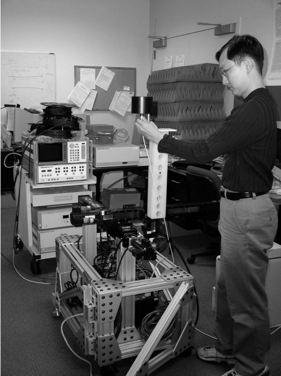
Figure 4. In the foreground, the actuator system and the antenna on the telescoping mast. Behind the actuator system is a cart holding the HP8530A microwave receiver and other components.
