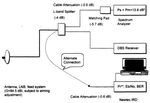
\* Pm is measured spectral density im 1 MHz. 13.8 = 10\*log (24 MHz, transponder flat bandwidth approx.) \*\* Pr = Ps+4+5.7 = Pm + 23.5 dBm
