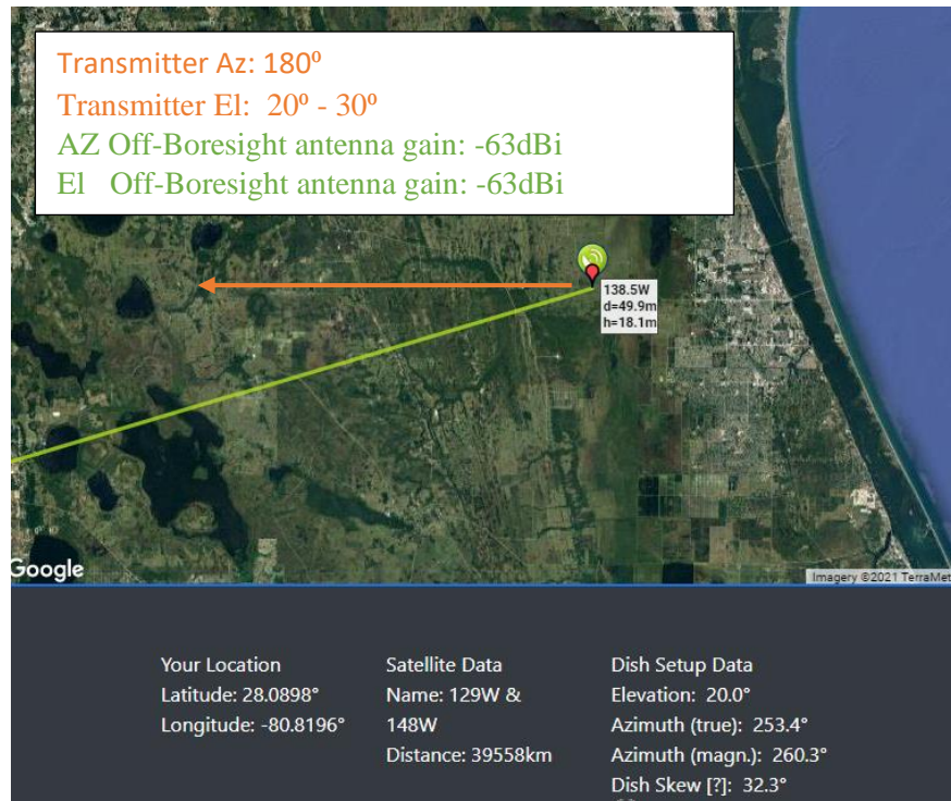
Figure 1. Test site azimuth pointing direction (orange) and off-axis pointing (green) towards GSO at 129°W
