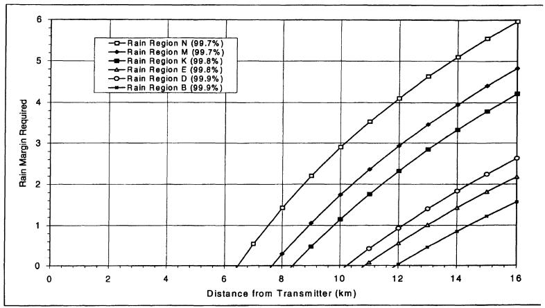
The rain margin required to meet specified availability accounts for both the lower rain attenuation and change in path loss over 16 km distance.
