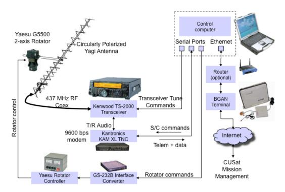
The antenna structure is one of the most important components in the ground station. Paired with a transceiver, it can single-handedly determine whether a radio connection to the satellite will be successful or not. An antenna also requires a rotator in order to correctly orient itself and point at the satellite. An incorrectly pointed satellite will have degraded quality of signal.
