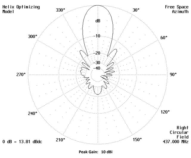
CAPTECHR SatNogs Helical Earth Station Receiving Antenna Radiation Pattern Diagram
