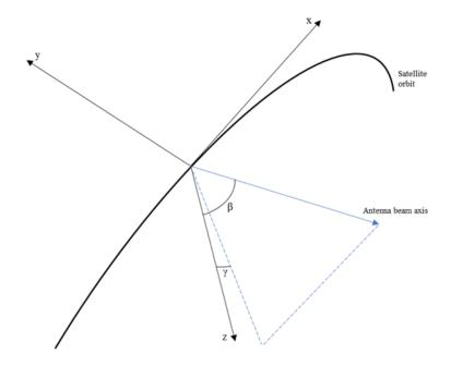
$\beta$  is the angle between the antenna beam and the z-axis  $\gamma$  is the angle of the projection of the beam axis onto the YZ reference plane, measured from the Z axis The range of possible beam angles are:  $\beta < 50^\circ$  and  $\gamma > 10^\circ$
