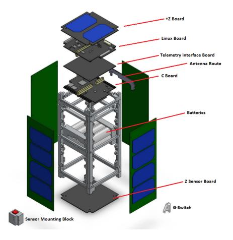
LEO will record vibrational and thermal measurements with two accelerometers and a thermocouple and also record vibrational data taken by a second CubeSat that will be transferred through WiFi during launch.
