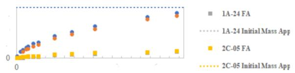
Figure shows sublimation mass over time - X axis is time and Y axis is sublimated mass. Due to sensitive information, units have been removed.
