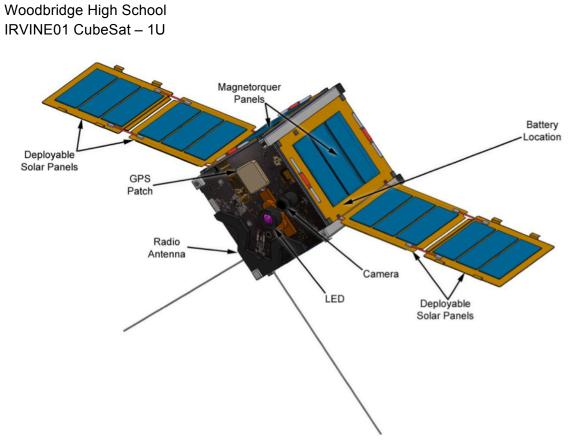
**Mission description:** Irvine01's main mission is to take pictures of the moon and planets and send them to the ground station where they will be used for educational purposes. The primary instrument is a 3 MP camera. In addition, magnetorquers will be used for attitude control, and solar panels will be used for power.
