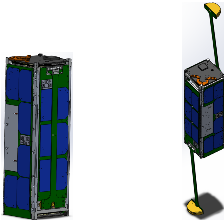
Figure 11: EXOCUBE Stowed/Deployed View
