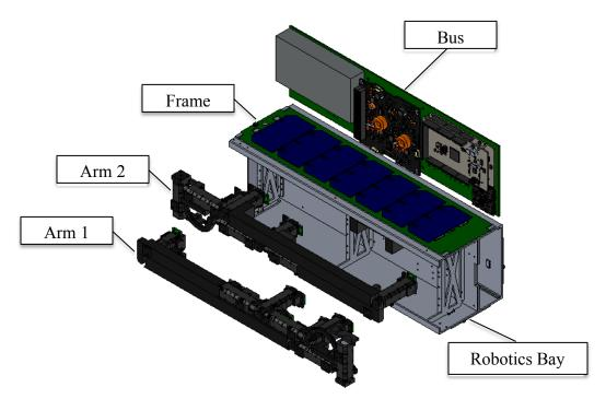
Figure 13: RSat Expanded View
