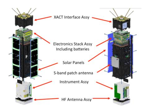
Figure 17: SHFT 3U Cube-sat Expanded View
