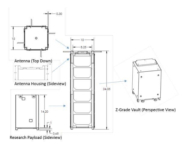
Figure 14: Shields-1 Expanded View
