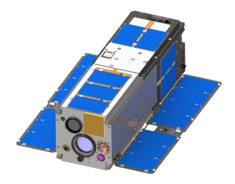
Figure 16:One of two AC11/TOMSat spacecraft with solar panels deployed.
