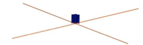
Figure 18: SHFT 3U Cube-sat Deployed view with 3 meter HF antennas
