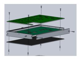
Figure 4: Sensor Node Expanded View
