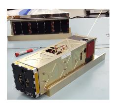
Figure 19: SHFT 3U Cube-sat Stowed configuration
