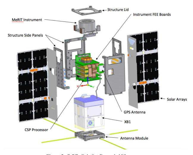
Figure 5: CeREs CubeSat Expanded View
