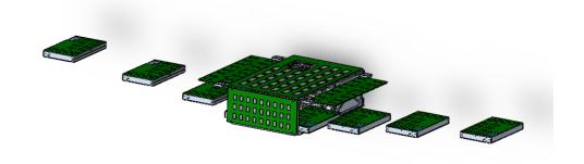
Figure 3: ANDESITE Sensor Node Deployment & Node Expanded View
