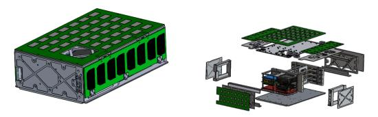
Figure 2: ANDESITE System and Expanded View
