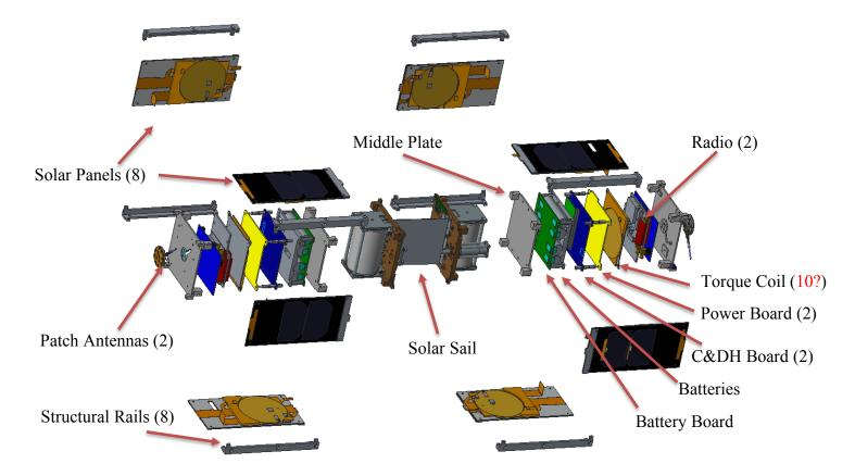
Figure 9: CubeSail Expanded View
