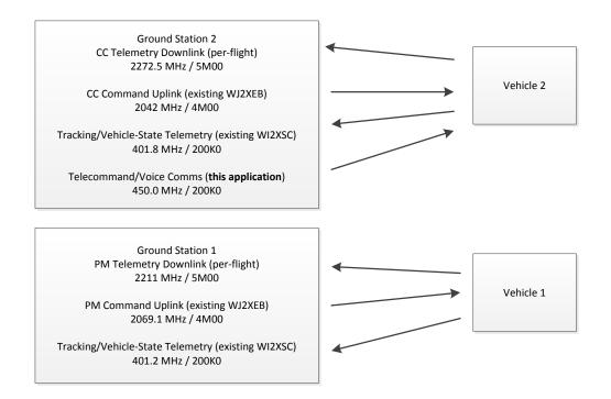
The telecommand and voice communications uplink system has the following characteristics:
