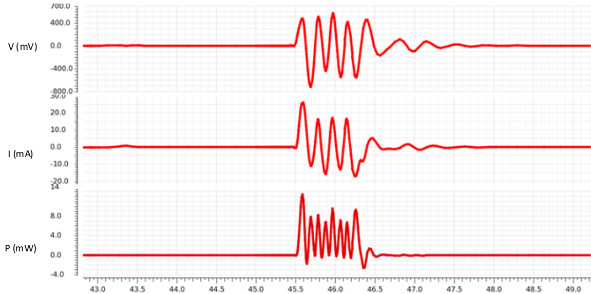
Figure 2. Simulated instantaneous voltage (V), current (I), and power (P) of a single pulse on implantable antenna input. P = V * I
