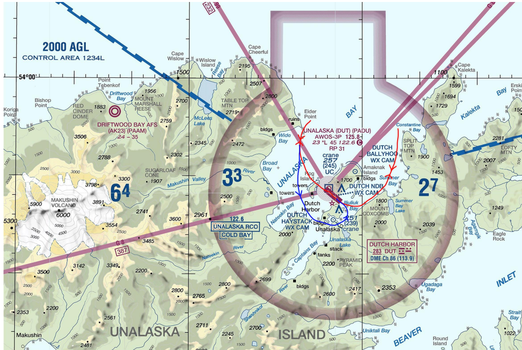
Figure – Map of airspace around DUT airport and Dutch Harbor. The thin red and blue traces drawn on the map show the typical arrivals and departures.
