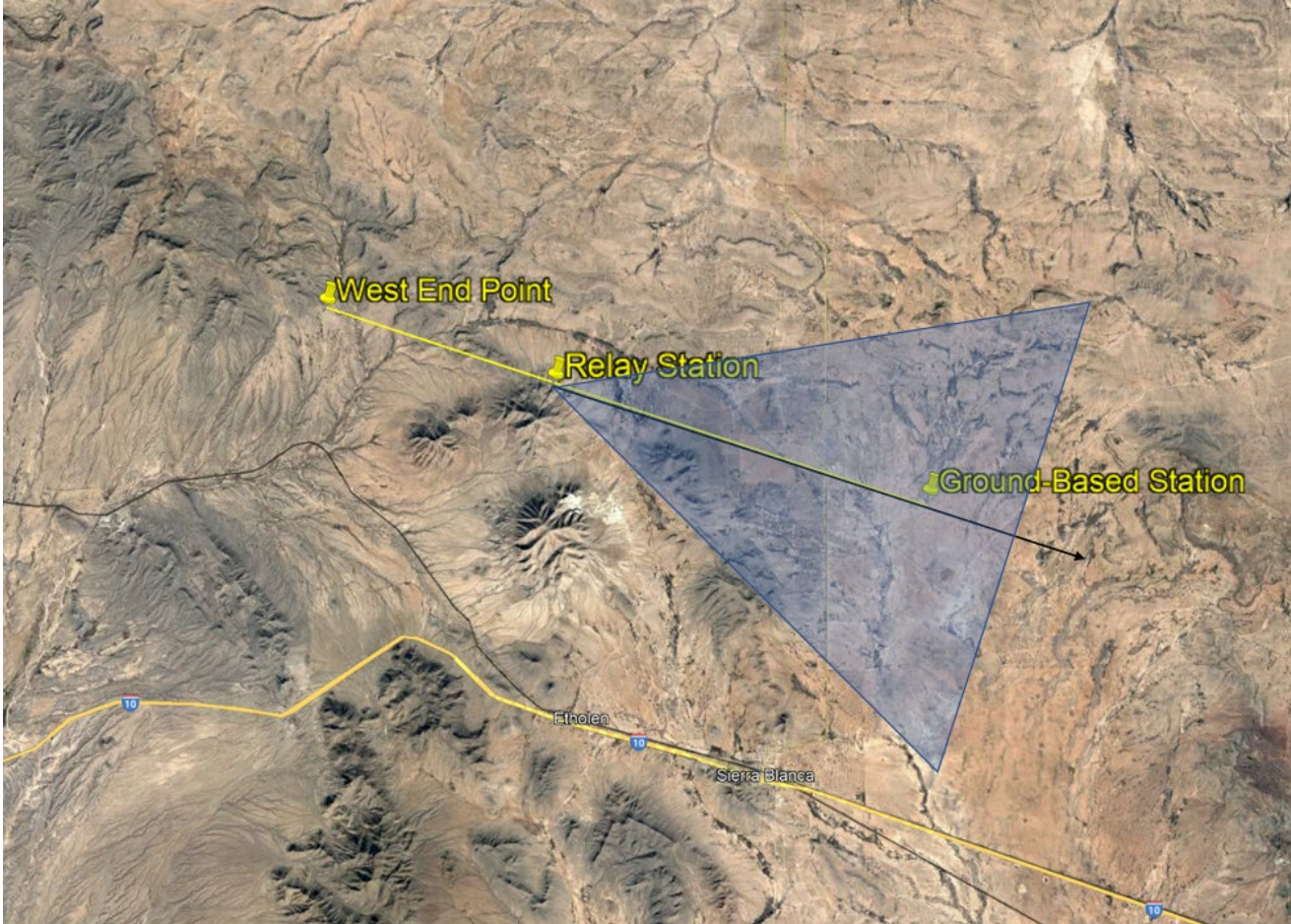
Figure 6: Graphical Depiction of Relay High Gain Antenna 3dB Coverage +/- 27.5 Degrees Off Center
