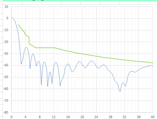
Antenna ESD Pattern: Uplink Elevation RHCP Low ESD (dBW/Hz) vs Azimuth Angle (degrees) 20190801m01v01.0_x135_AntennaPlots.xlsx XlowRHCPulei
