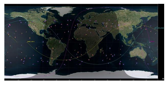
In a one year time period, the closest approach experienced between RROCI and the ISS is 28.9 km, with a mean range of 159.9 km when inside the 200km limit. The closest approach between RROCI and the Chinese Space Station is 18.6 km, with a mean range of 170.9 km when inside the 200km limit.
