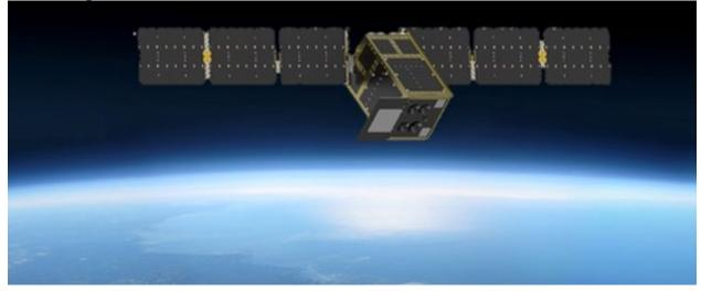
The solar panels rotate around an axis perpendicular to the velocity vector, as shown in the following figures.
