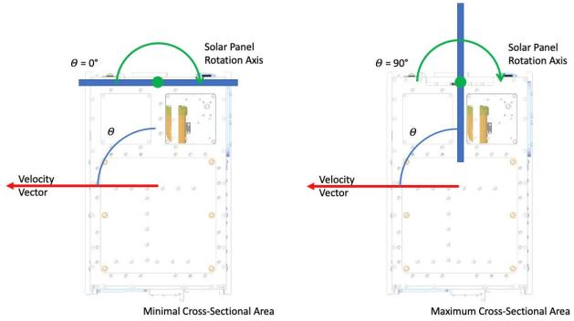
By modifying the angle of attack into the velocity vector direction, we can modify the drag profile of the spacecraft system. The mission will already perform this angle modification maneuver multiple times per orbit to track the sun and maximize the solar power generation for the system.
