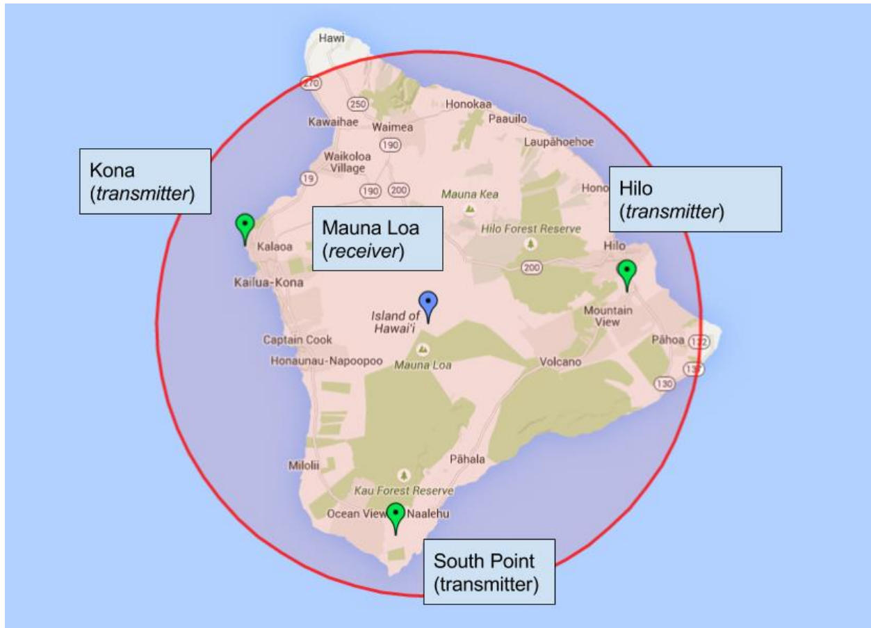
Figure 3: Proposed transmitter locations (green pins) and the receiver station (blue pin). The red circle represents a 75 km radius from the receiver, which is suitable for measurements made by the TIDDBIT system.
