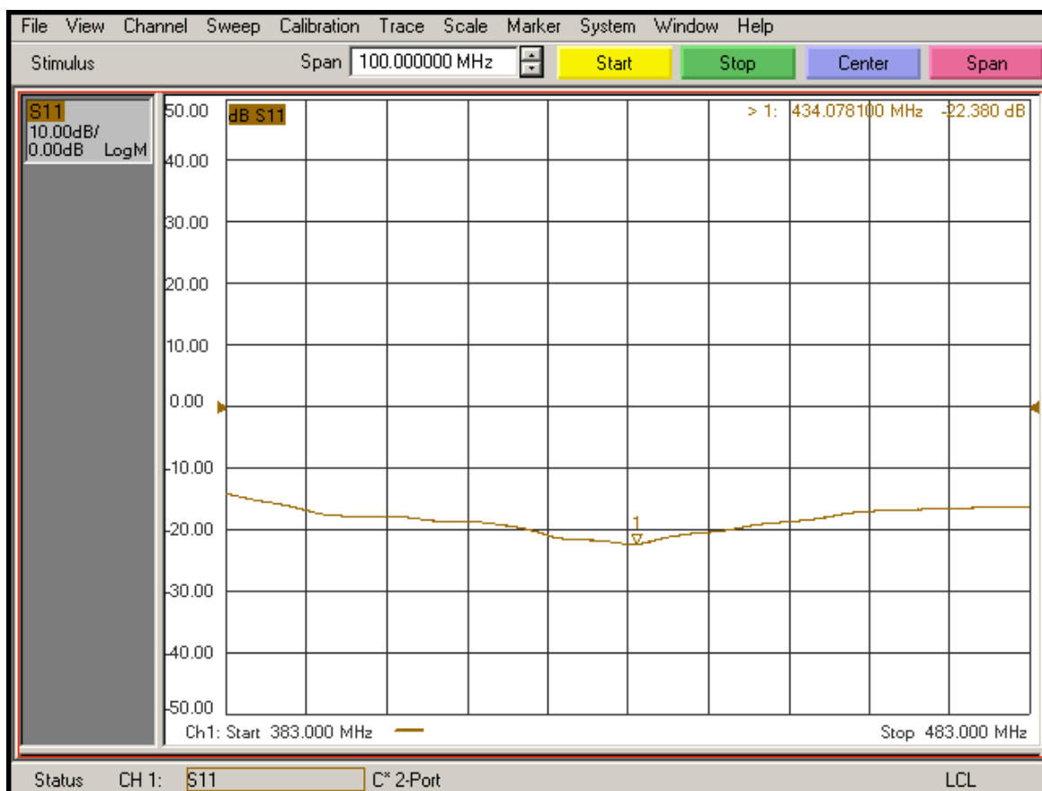
Figure 5 - measured return loss of the UHF antenna
