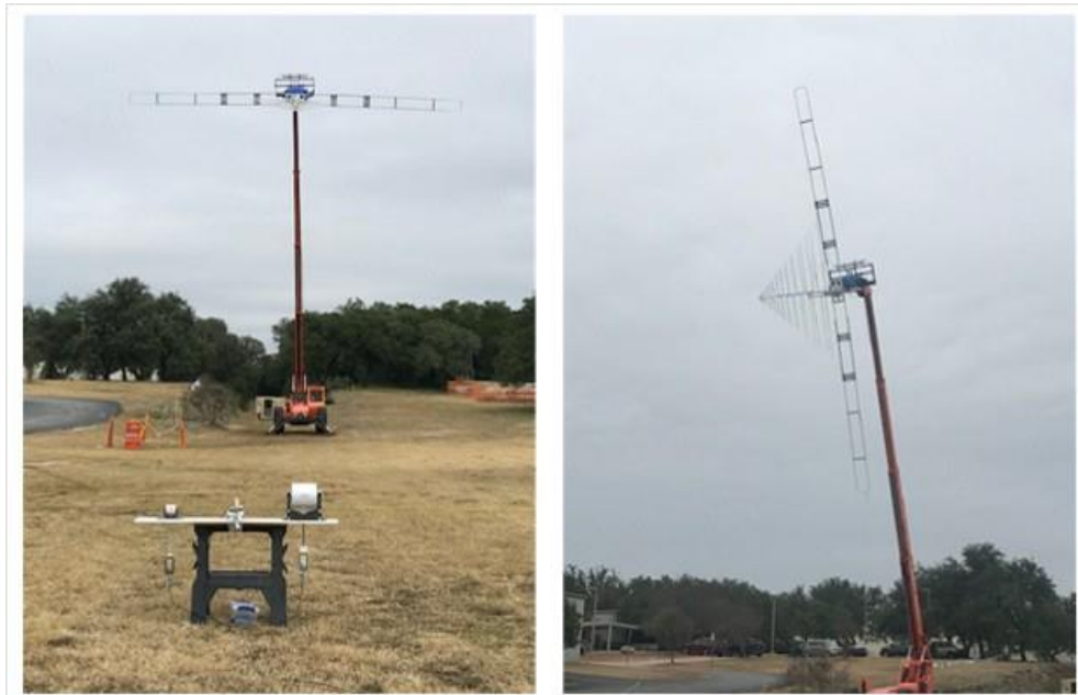
Figure 3: Proposed CWI Antenna System Mounting Scheme (Telehandler Height Maximum 55ft.)
