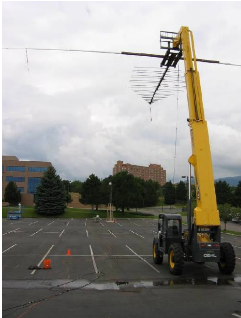
Figure 4. Proposed CWI Antenna System Mounting Scheme (Telehandler Height Maximum 55ft.)
